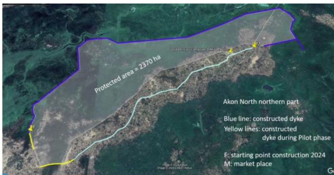
Figure 4 Phase 1 Dike to be repaired, reinforced and topped-up to the safety level standard (18.5 km)
